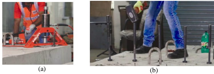
Figure 4. (a) Torsion-controlled hydraulic pullout tester. (b) Crack generation in the line of anchors with the help of steel wedges
